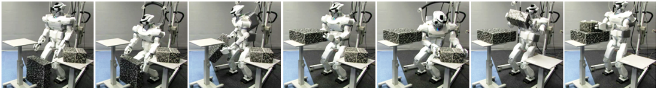
Figure 8.8: Snapshots from the execution of the box stacking task on the HRP3 robot.
