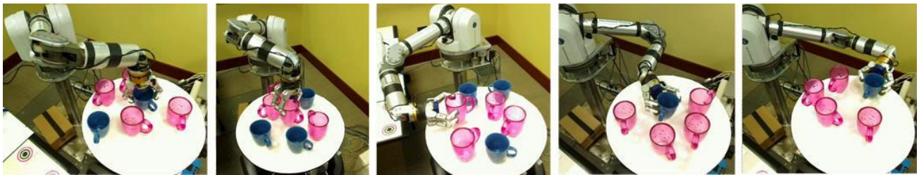
Figure 15.10: The robot grasping blue and red mugs in various scenes. In the three right-most pictures an artificial obstacle was added above the mugs to make the problem more difficult.
