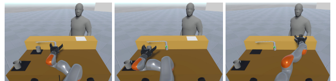
Fig. 9 Multi-stage simulated manipulation task: first fill the cup, then grasp it, and then deliver it. To avoid spills, a pose constraint is enforced after the cup is grasped.
