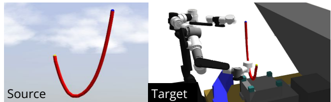
Fig. 3: Source environment for bimanual rope manipulation (left) and simulated target environment (right) where there is a robot, obstacles, and the rope damping and stiffness are changed.
