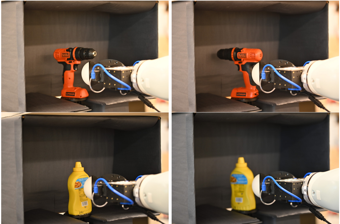
Figure 4.3: Real probing configurations for the drill and mustard.
