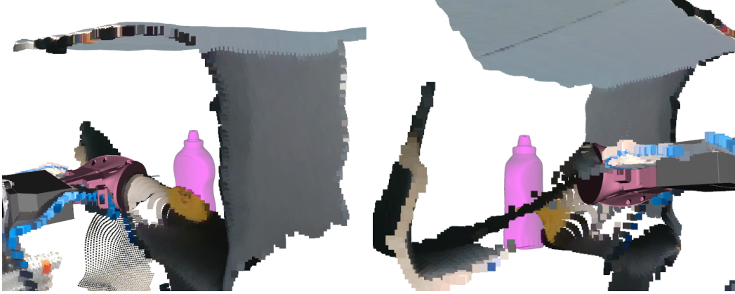
Figure 4.5: Unreliable RGBD readings inside the partially occluded cabinet, viewed from both sides, with an approximate pose of the mustard bottle in purple.
