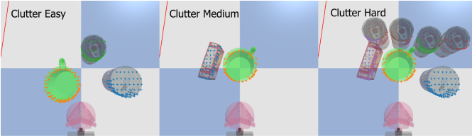
Fig. 15: Starting configuration of clutter experiments with clustered surface points rendered in different colors. All objects are movable and the mug is the target object. Clutter Medium may appear simpler than Clutter Easy, but due to the closer proximity of the objects, it becomes a more difficult task.
