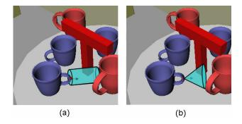
Fig. 3. Depiction of computing distances to obstacles for one point on an object using cones and cylinders. The cone/cylinder is oriented along the outward-facing surface normal of a point on the surface of the object. The length of the longest cone/cylinder that is collision-free is the distance score assigned to that point.
