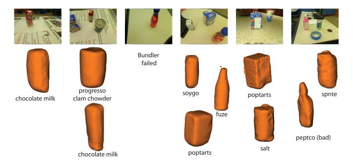
Fig. 4. Reconstructed models follow the shapes of the objects well. Visible defects are caused by (1) low camera resolution (640x480) (2) limited visibility at contacts with the table (3) featureless regions (peptco, duck tape), (4) non-planar and specular surfaces (e.g. sprite can)
