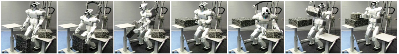
Fig. 6. Snapshots from the execution of the box stacking task using the HRP3 robot.
