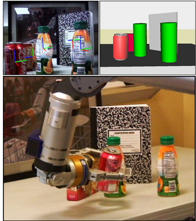
Fig. 1. Object grasping in a cluttered scene through pose estimation performed with a single image. (top left) Scene observed by the robot's camera, used for object recognition/pose estimation. Coordinate frames show the pose of each object. (top right) Virtual environment reconstructed after running pose estimation algorithm. Each object is represented using a simple geometry. (bottom) Our robot platform in the process of grasping an object, using only the pose information from this algorithm.
