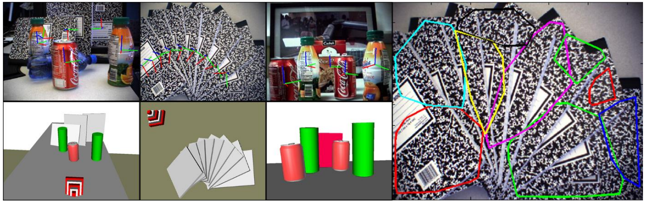
Fig. 6. The importance of clustering in cluttered scenes. The camera position is represented as a red and white pyramid. (Col 1) Scene with 1 soda can, 2 juice bottles and 3 notebooks. The water bottle is not an object in the database, and is therefore only treated as another occlusion. Note that the notebook on the right is upside down, and correctly detected. Without Mean Shift, this scene requires 121 iterations of RANSAC. With Mean Shift, it requires 38. (Col 2) Scene with 9 highly-occluded notebooks. Without Mean Shift, the algorithm is only able to find 6 notebooks before the 3000 iterations limit is reached. With Mean Shift, 9 clusters are formed and all 9 notebooks are detected -with no outliers- after 454 iterations. (Col 3) Scene with 2 soda cans, 2 juice bottles and 1 rice box. Without Mean Shift, 115 iterations. With Mean Shift, 33 iterations. (Col 4) Clusters of correspondences in Notebooks image.
