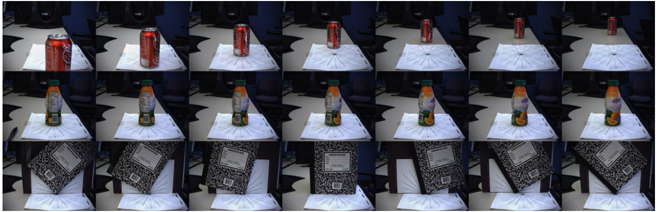
Fig. 5. Examples of the different experiments run on the accuracy test. (Top row) Coke can translation test. (Middle row) Juice bottle out-of-plane rotation test. (Bottom row) Notebook in-plane rotation test.
