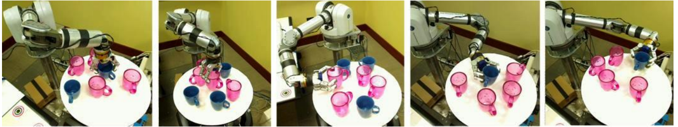
Fig. 11. The robot grasping blue and red mugs in various scenes. In the three right-most pictures an artificial obstacle was added above the mugs to increase difficulty.
