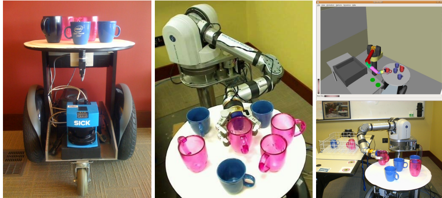
Figure 1. The Robotic Busboy composed of a Segway RMP200 and a Barrett WAM arm, with a snapshot from simulation and reality.
