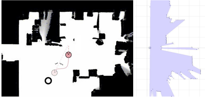
Figure 4. Laser-based obstacle avoidance. A person stands between the segway and its desired location. The person is detected by the Segway’s laser range finder and is avoided.
