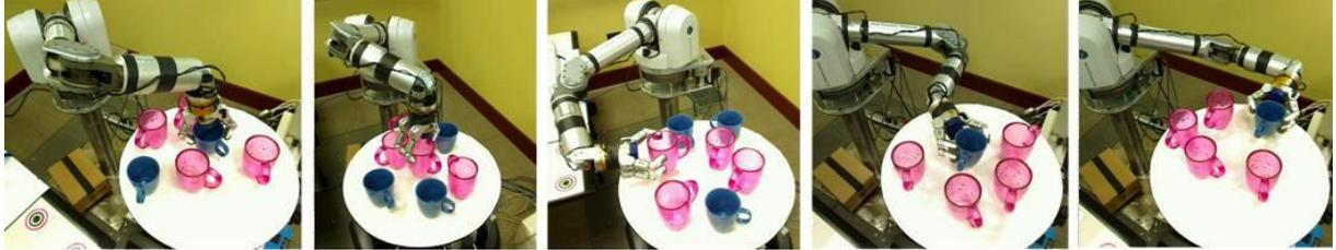
Fig. 8. The robot grasping blue and red mugs in various scenes. In the three right-most pictures an artificial obstacle was added above the mugs to increase difficulty.
