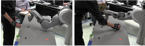
Fig. 9. A comparison of robot configurations generated by the baseline method (left) and the avoidance-only method (right). The baseline method is occluding the human's goal region while the avoidance-only method leaves the goal region open.
