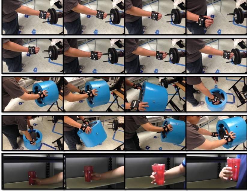
Fig. 3. Snapshots from humans demonstrating the five tasks. We only use the poses of the moving object and the reference object in our method. From top to bottom are remove nut, insert nut, unhang tire, hang tire and retrieve cup, respectively.
