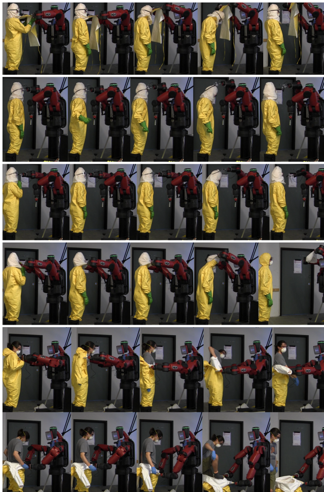
Fig. 4: Robot-Assisted doffing using transfer motions. Top-to-bottom: Apron, Goggles, Faceshield, Hood, Coverall.
