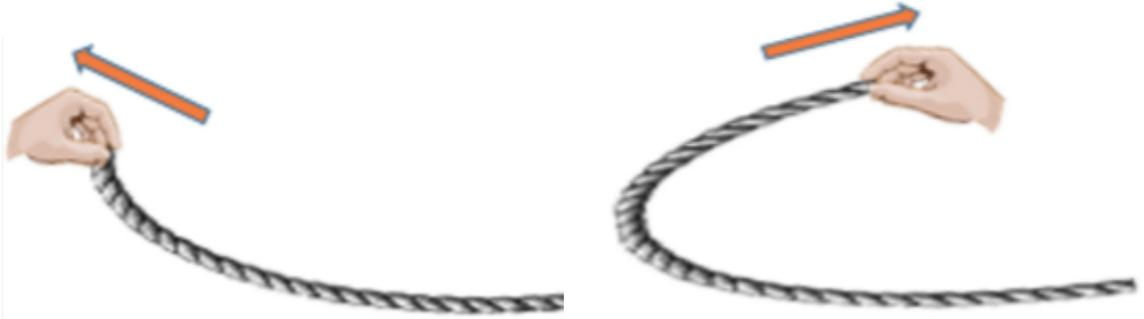
Figure 3.2: An illustrative example of directional rigidity. Left: The rope moves almost rigidly when dragging it by one end to the left. Right: The rope deforms when pulling it on the right in the opposite direction.
