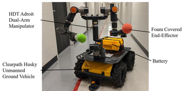
**Fig. 11** The mobile manipulator used in the experiment. The end-effectors are padded with foam covers to reduce damage on the surface of the end-effector when making contacts
