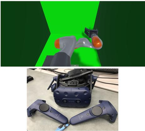
**Figure 16.** VR setup. **Top:** VR environment. The green box represents the position constraints. The end effector is commanded to move by selecting and dragging to a desired position with the HTC Vive controllers. **Bottom:** Vive hardware.
